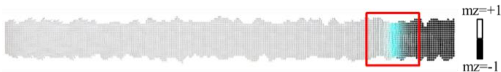
Figure 3-8 A rectangular region of dimension 60 \times 50 \times 1 \text{ nm}^3 marked in red is centered around the DW in a racetrack. The energy densities are calculated for the red rectangular region by changing the cell sizes of the simulation. The computed energy densities are shown in table 3-2.
