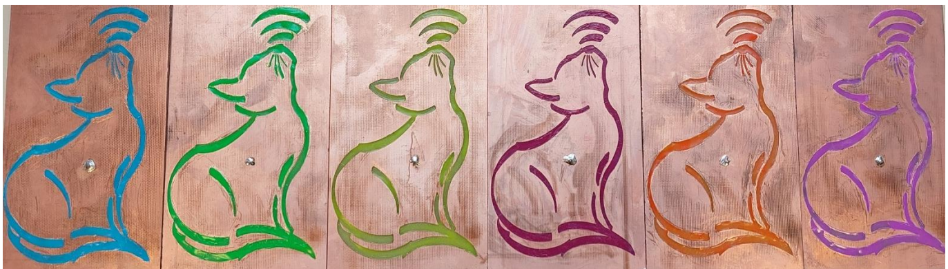
Figure 46 Six versions of epoxy-treated AntennaCAT logo cat-shaped antennas used for validating optimizer results.
