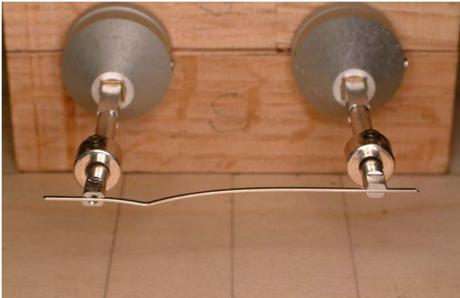
**Figure 7.** 2-Dimensional model: Measuring moments and forces.
